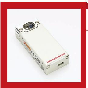
MEMS-FPI spectroscopic module C17552 / C17553 / C17554 This compact module has a bult-in light source, control circuit, and MEMS-FPI spectrum sensor and MEMS FPI tunable filter which can vary its transmission wavelength by changing the applied voltage.
