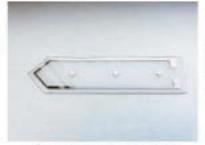
Thermocouple element formation on plastic film
