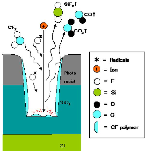
Fig. 3 Reaction model of during dry etching of dielectric materials.
