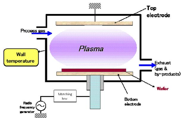
Fig. 4 Etching chamber.
